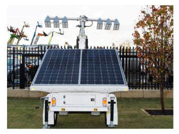
Welcome to the future of mobile lighting, the LTA Solar 65K. Generators Australia has a new lighting tower that is run solely by renewable energy.
